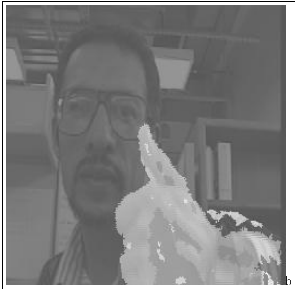
Figure 8: MAP motion-based segmentation algorithm. (a) Segmentation field e of hand # 1 . (b) Superposition of frame 3 of hand # 1 and segmentation field e .
